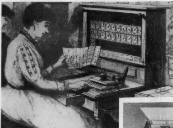
The first die-set punch, developed by Powers for the census of 1910. The operator set up on the keyboard all the values to be punched; she then used the knee-treadle to gang-punch the card.
